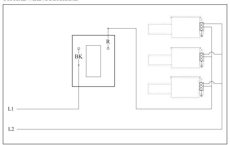
Up to 3 line voltage tube heaters or multiple line voltage DR heaters can be wired to this thermostat.
